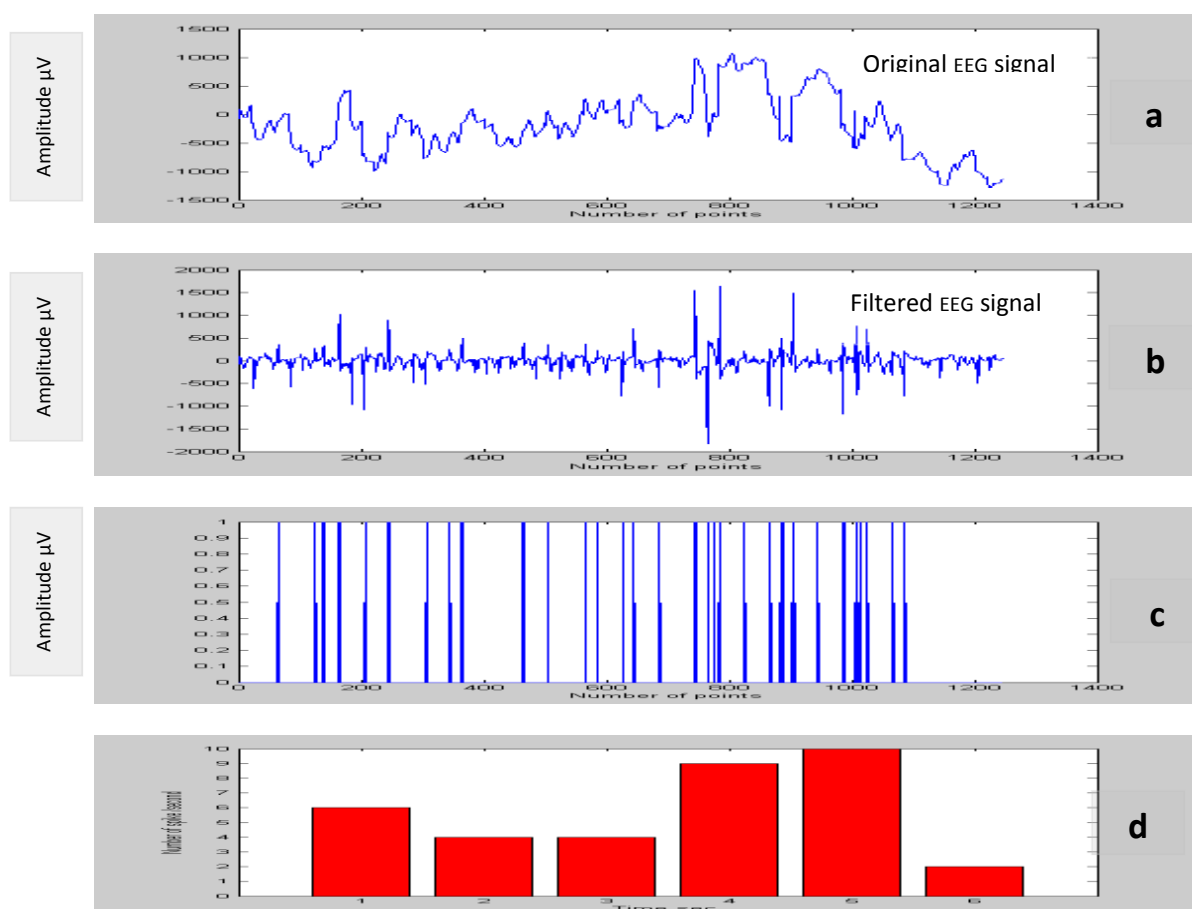
Figure (20): (a) Original record for one minute of EEG record on channel two for normal subject (b) the signal after being filtered with the digital filter whose z-plane is shown on figure (15), (c) the point process representation of the spike sequence (d) spikes per second bar chart
