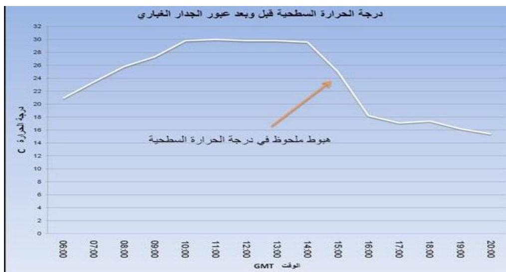
Figure (15) Temperature measurements during dust storm
